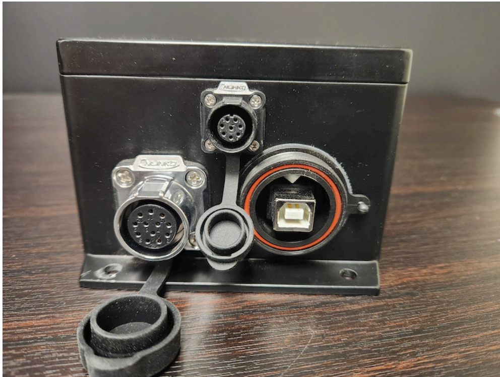
Figure 1. SpraySync WT1 Monitor Box Inputs
