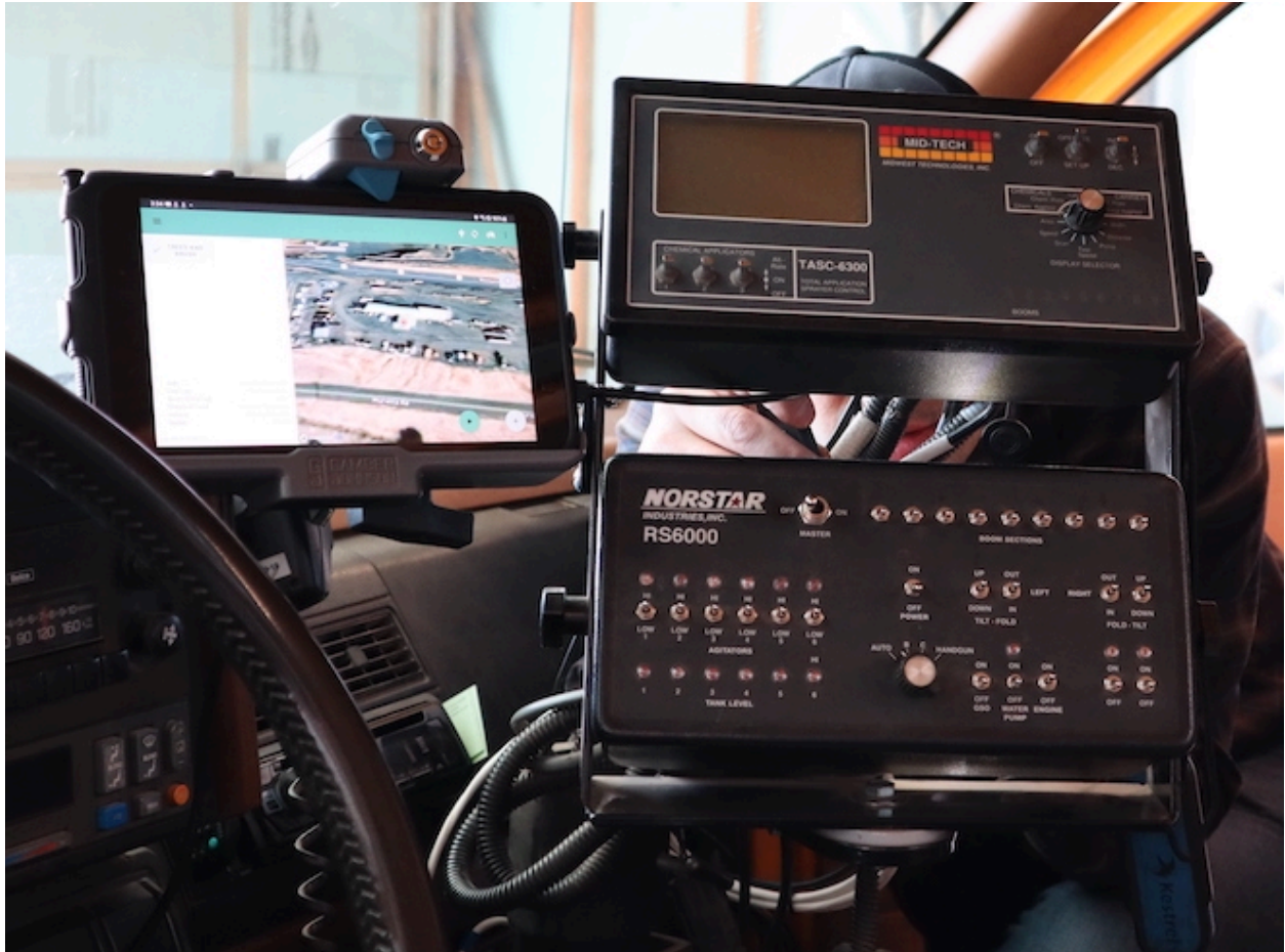
Figure 24: Norstar RS6000 with Tablet mount installed
