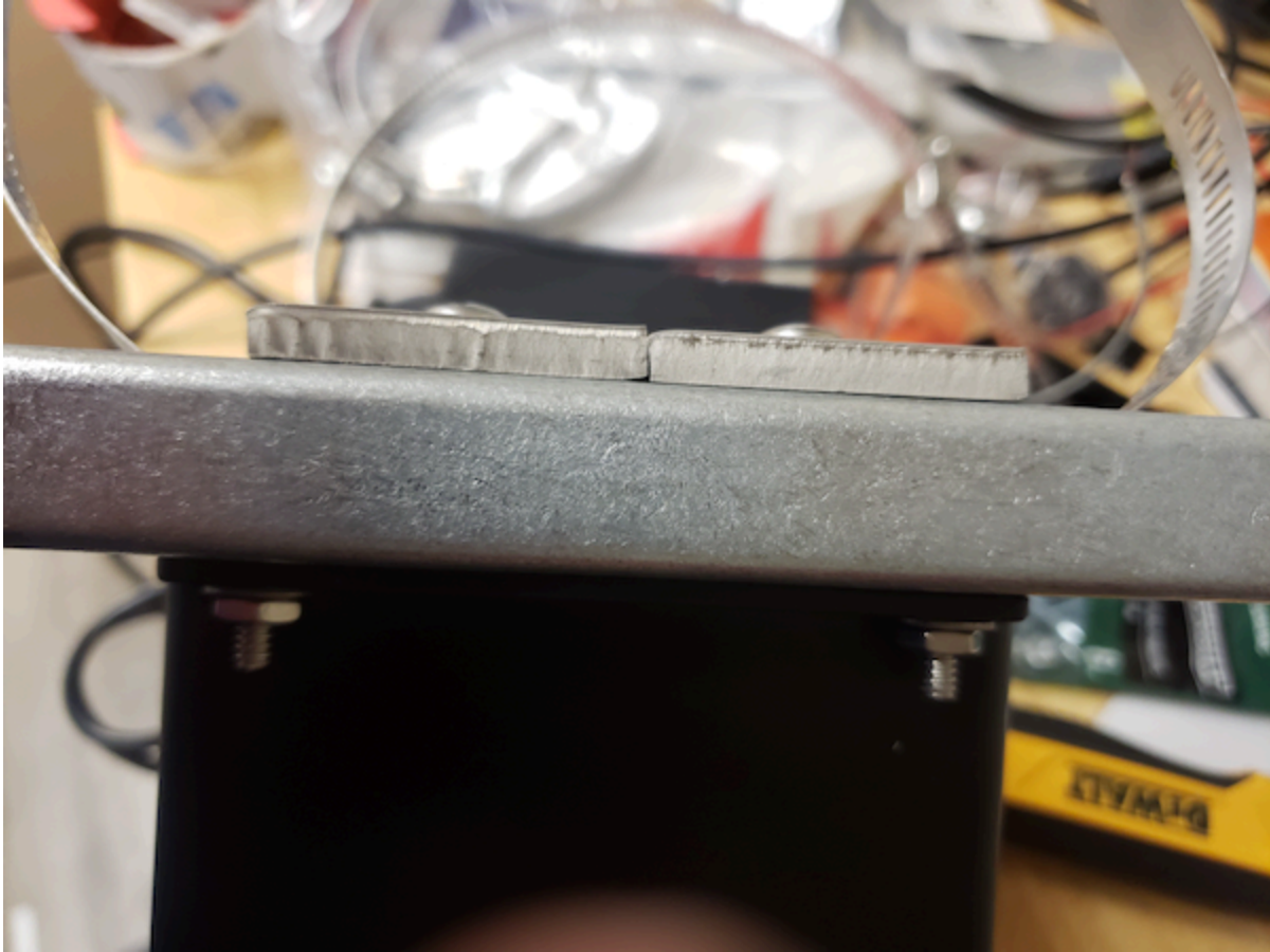
Figure 19. Closeup of pole mount kit bolted into monitor box flanges.
