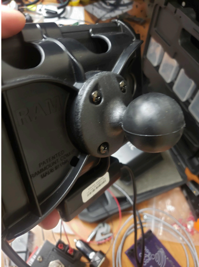
Figure 28: Tablet mount with ball mount plate attached
